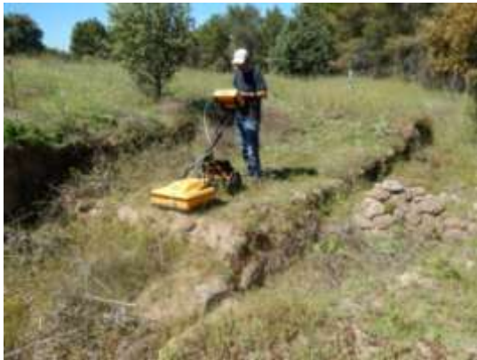
Application of 2D Georadar to the Cerro de la Mesa (Toledo) site and of the 600 MHz multi-channel Georadar antenna in the Visigoth necropolis at Ermita de la Vega (Guadalajara)
