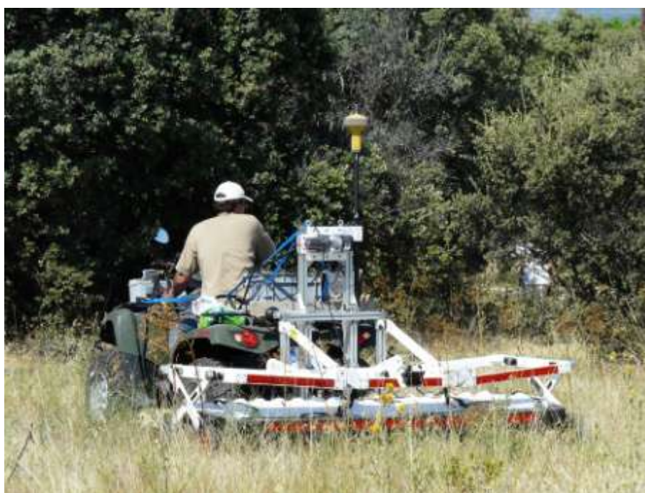
Application of multi-channel georadar with 200 MHz antenna and differential GPS in the area of the dolmen at Entretérminos (Madrid)
